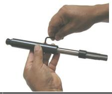
The reamer will also cut the Countersink for the flange of the insert to seat into. When you start getting close to the stop collar coming in contact with the head, you will want to clean the chips from the reamer so you have a positive stop on the head without having any chips interfering.
