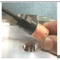
**B:** Lightly tighten the socket cap screw.
