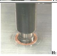
Remove driver, repair is complete.
