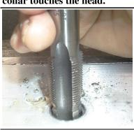
Mechanics Tip 1: Packing the flutes with grease will help to catch any stray chip from going into the cylinder.
