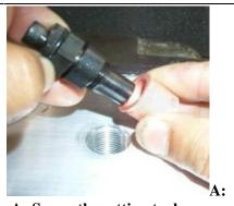
**A:** Screw the setting tool into the insert.
