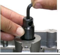
4) Insert driver tool Oil the bottom threads of the driver picture G: Screw the driver into the insert you will feel the driver start to tighten up. Use a little more power and continue through the insert. Do not let the larger diameter of the driver shank hit the insert.
