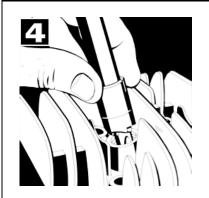
4. Using the wrench provided rotate the seat cutter. After a few turns lift the seat cutter to inspect the seat. Repeat operation until the seat is completely cleaned up. Remove the step tap from the hole.
