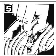
Make sure the hole is clean and dry. Lubricate the driver tool with Time-Sert driver oil or 30 wt motor oil. Screw an insert into the prepared hole.
