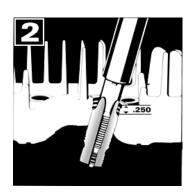
Using the wrench provided place wrench over tap and tap new threads. Continue to tap through until the cutting edges are approximately 1/4" inch or 6mm below surface.
